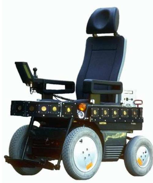
Fig. 3. The autonomous wheelchair Rolland that was model-checked for mode confusion problems.
